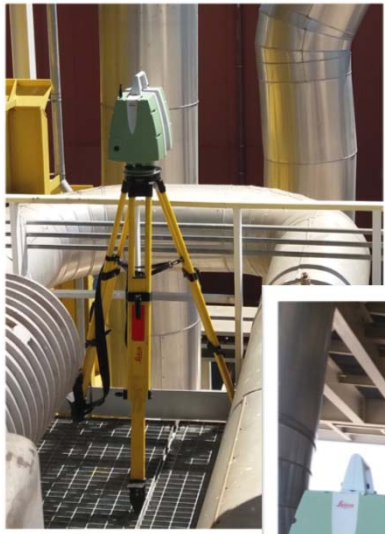
3D Laser Scanner Leica P20, view 360° x 270° and cloud of 1.000.000 point to second
