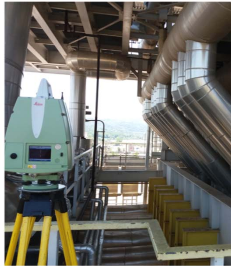
3D Laser Scanner Leica P20, view 360° x 270° and cloud of 1.000.000 point to second
